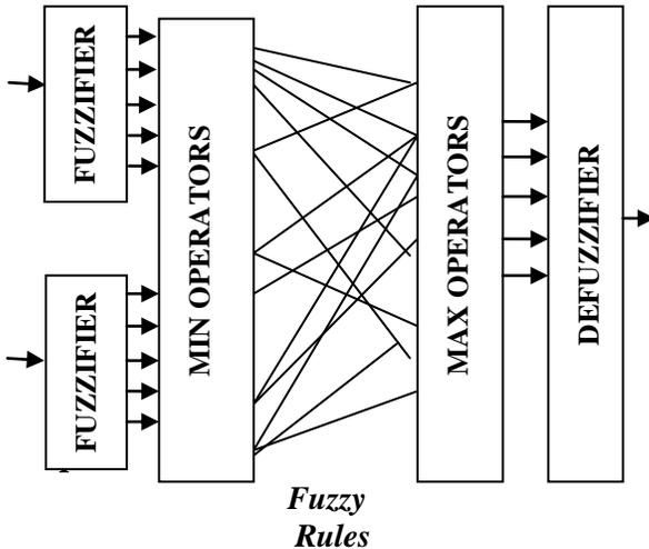
Fig. 3 Block Diagram of Fuzzy System
